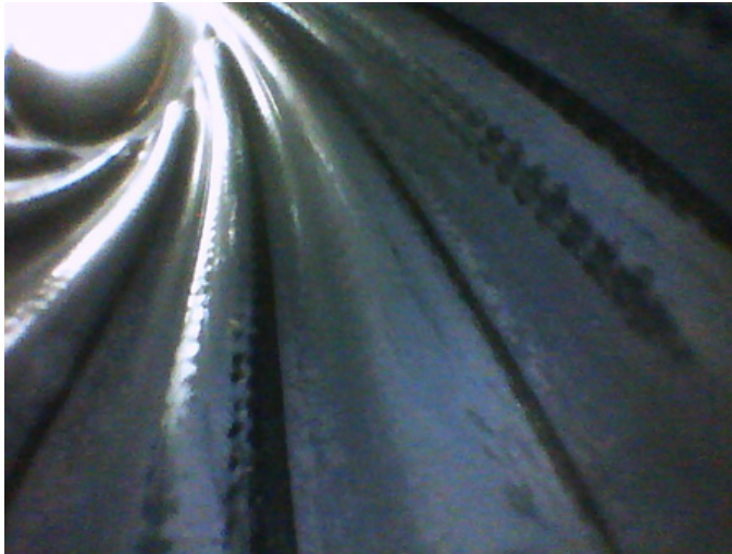
Figure 4 - Post-run borescope of stator
