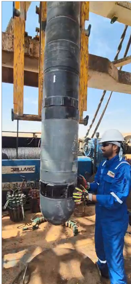
13-3/8" HSRT: Hi-Speed Reaming Tool prior to surface test.
