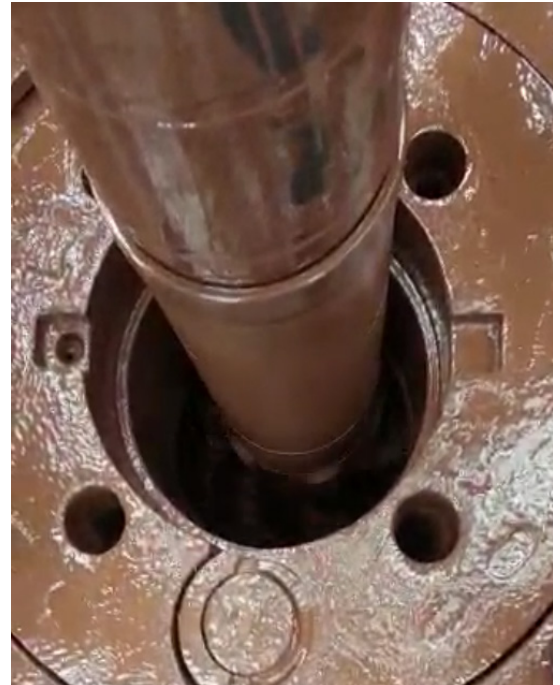
Surface testing the 9-5/8" HSRT prior to starting the casing run.
