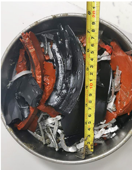
Aluminum cuttings recovered while the 9-5/8" HSRT was being drilled out.
