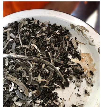
Aluminum cuttings recovered while the 9-5/8" HSRT was being drilled out.
